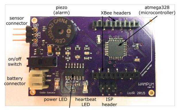
quad op-amp IC (filtering & amplification)
